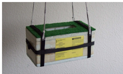
Fig. 1: The disdrometer Flying Parsivel. The overlay of synthetic turf prevents drops from splashing on the housing and contaminating the measurements.
