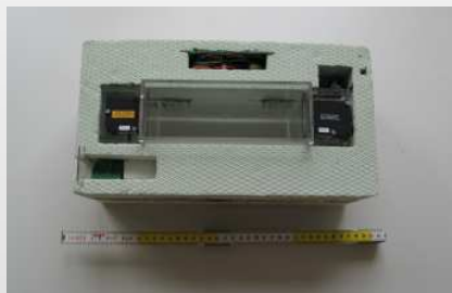
Fig. 2: Opened Flying Parsivel. The laser light sheet is located in the core of the housing.
