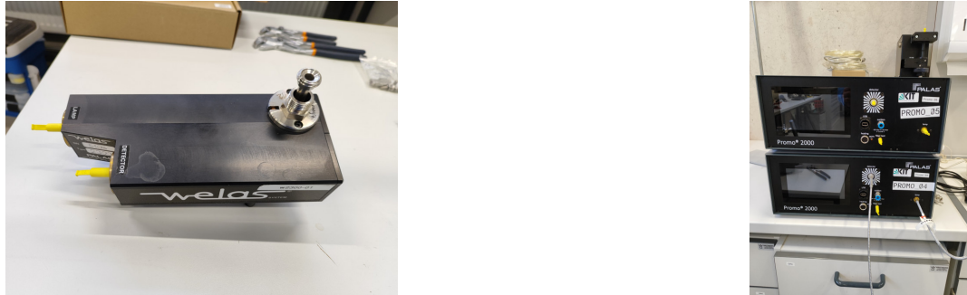
Figure 2.11.: Pictures of a welas sensor (left) and the Promo devices used in the HyICE23 campaign (right)
