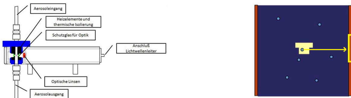
Figure 2.12.: welas sensor, schematic of structure of the sensor (left) and schematic working principle (right)
