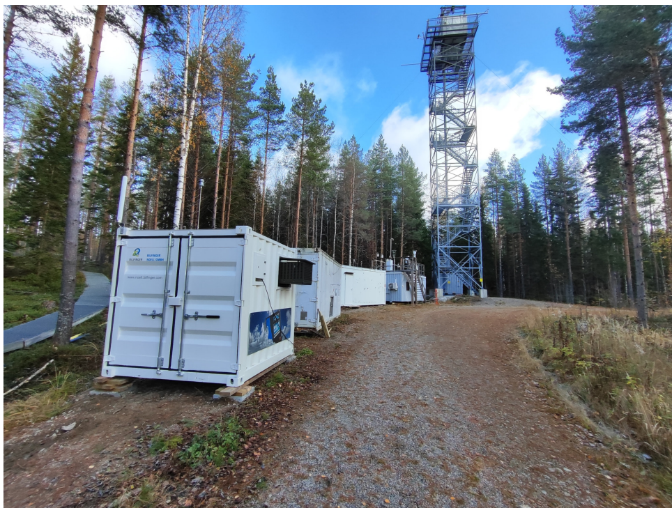
Figure 3.2.: Picture of the PINE container and the 35 m tower of SMEAR II. On top of the PINE container on the left, the PM 10 inlet (Comde-Derenda) is visible. The same inlet was used for the filter-based measurements on the tower.
