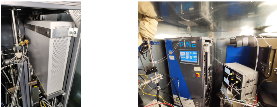
Figure 3.5.: Pictures of the additional welas-2500 sensors and Promo-2000 devices added during phase 3. A picture showing a welas sensor built into the PINE instrument (left). The welas sensor built in before the split of the sampling line and the Promo devices are shown on the right.
